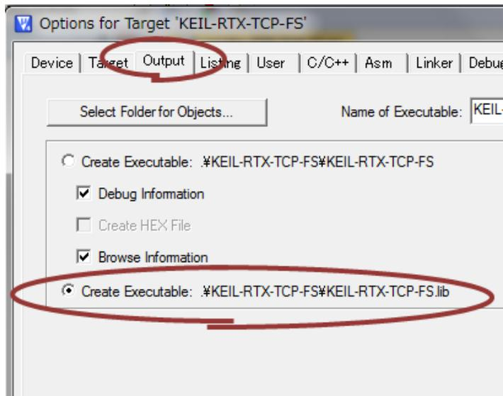
Select "Project" -> "Rebuild All Target Files" and get the \*.lib file under the build folder.
