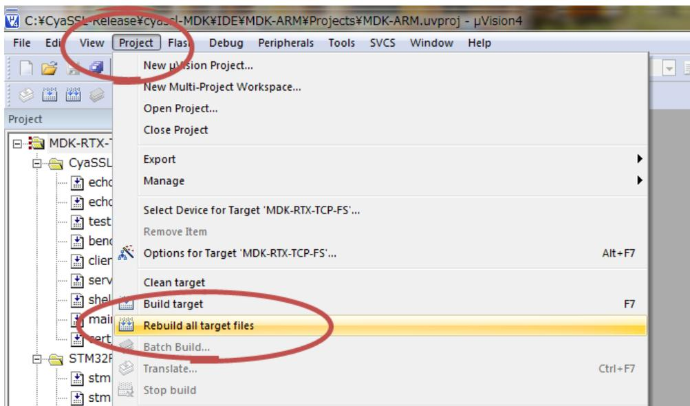
The compiled target file contains CyaSSL, MDK-RL (RTX, TCPnet and FlashFS), test apps and a tiny shell for invoking the apps through the PC keyboard.
