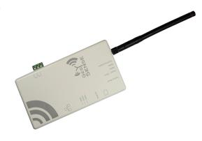
The GesySense Receiver \LAN Device
